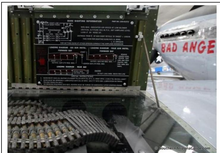
**One of "Bad Angel's" .50 caliber machine guns built into its wings.**
